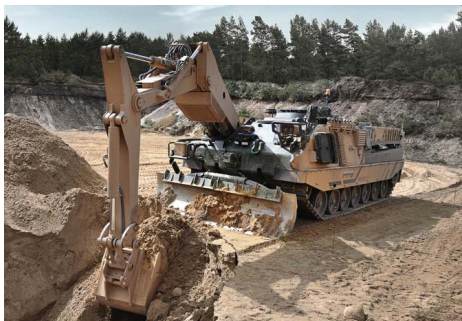
WISENT 2 operating in its armored engineer vehicle configuration
